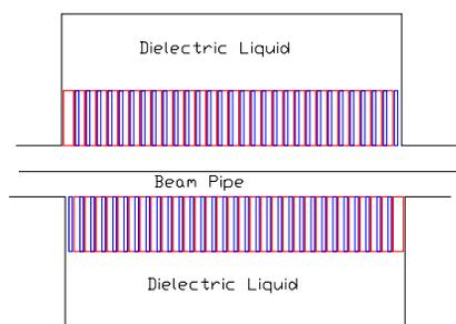
Figure 3: Dielectric Loaded Cavity for Phase Rotation
