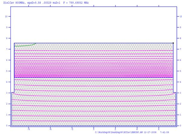
Figure 2. SuperFish output for 800MHz cavity with ceramic insert and short drift tube
