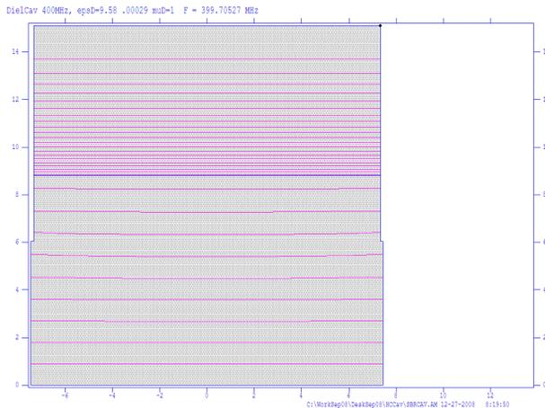
Figure 1: 400MHz cavity with dielectric insert.
