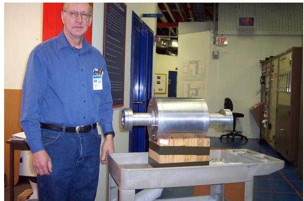
Figure 7: Model RF showing the moveable sleeves that allow the separation of the irises to be changed.
