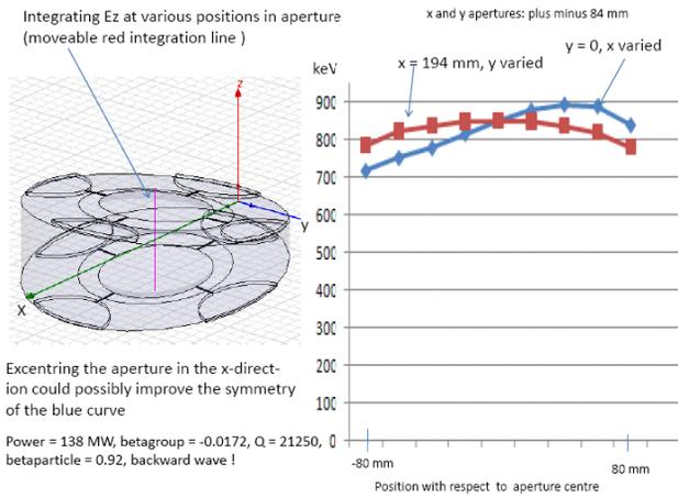
Figure 5: Integrated single-cell acceleration field variation.
