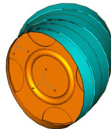
Figure 4: Hybrid travelling wave cell with forward (single central opening) and backward (4 peripheral openings) for power coupling, yielding a reduced net RF power flux.
