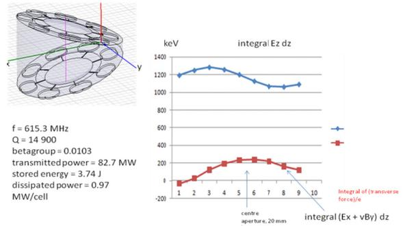
Figure 8: 615 MHz single-cell: integrated acceleration and transverse kicks in the x-direction.
