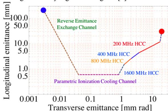
Fig. 1: Fermow-Neuffer plot of emittance evolution for a muon collider. Dashed lines represent parts yet to be simulated, solid lines are simulated with realistic magnetic fields generated by practical current conductors but not practical RF solutions.
