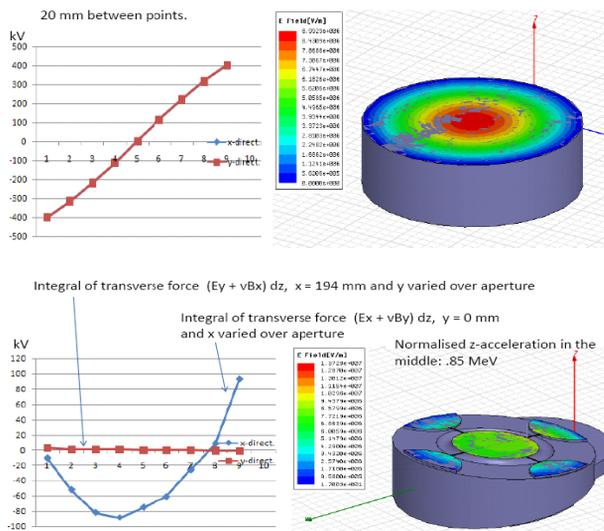
Fig.6: Comparison of integrated transverse kicks between a cylindrical pillbox [top] and the wedge shaped cell (containing a small asymmetric alcove to reduce the kick in the x-direction at the aperture middle. Offsetting the beam aperture with respect to the cell wall does the same).
