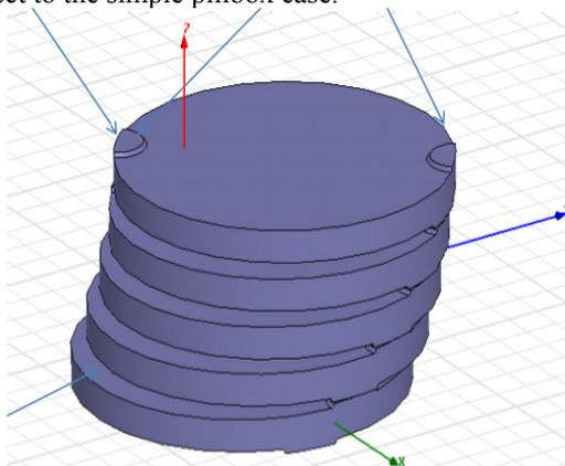
Figure 3: Backward-wave structure oriented in the helix axis direction.
