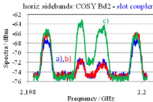
Figure 4: Horizontal betatron sidebands measured with a) new slot couplers (blue), b) COSY  $\lambda/4$  structures with aperture 90 mm, c) with aperture 40 mm
