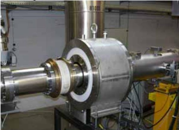
Figure 7: The barrier bucket cavity with its asymmetric layout is installed in one arc of COSY. In this figure, the shielding of the gap is dismantled to make it visible.
