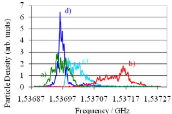
Figure 8: Schottky spectra of COSY beam measured at the 1000th harmonic: a) starting distribution, b) final distribution after 160sec only pellet-target, c) final distribution with longitudinal stochastic cooling and d) final distribution with cooling and barrier bucket.
