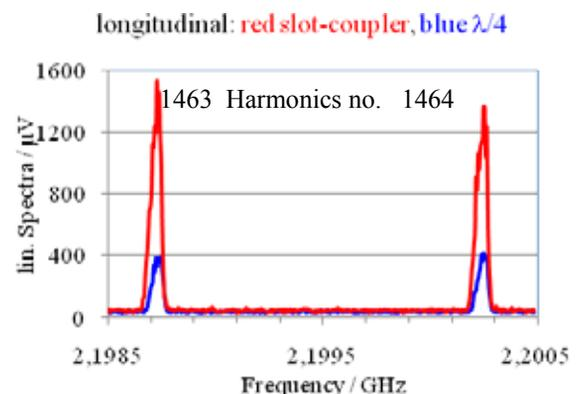
Figure 2: Harmonic number 1463 and 1464 of a 2.2 GeV/c proton beam measured with new slot couplers and new  $\lambda/4$  structures.
