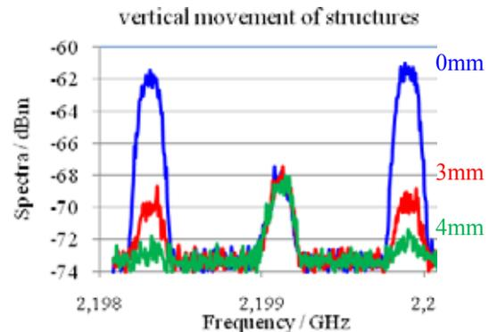
Figure 5: Minimizing longitudinal parts in transverse mode by moving the structures.
