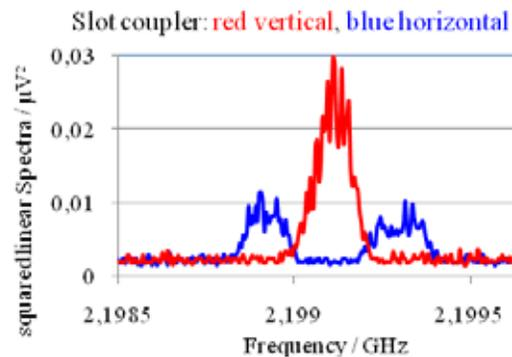
Figure 6: Vertical and horizontal sidebands measured with the same slot ring structure: no coupling was found.
