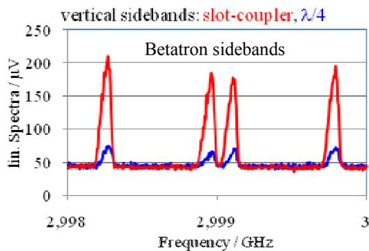
Figure 3: Comparison of transverse sensitivities between new slot ring couplers and new  $\lambda/4$  structures.
