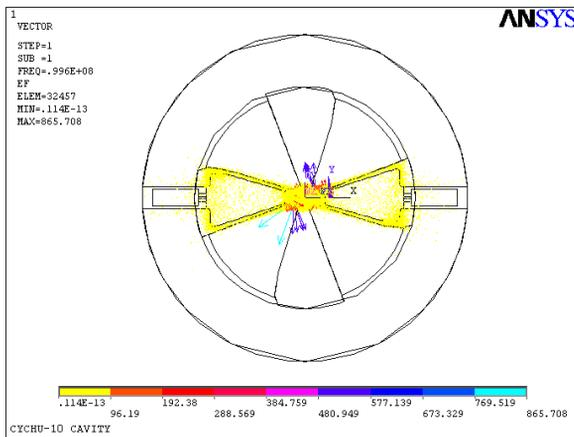
Figure 2: Electric field distribution
