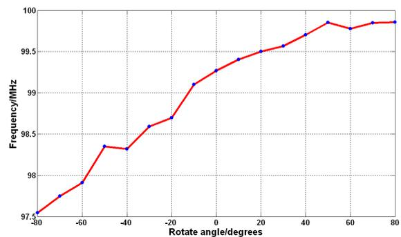
Figure 5: Trimmer compensation frequency range
