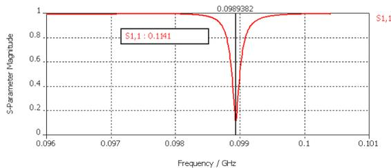
Figure 7: Reflection coefficient S11
