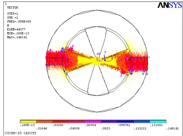
Figure 3: Magnetic field distribution
