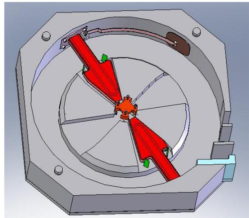
Figure 1: Horizontal  $\lambda/2$  coaxial resonance cavity
