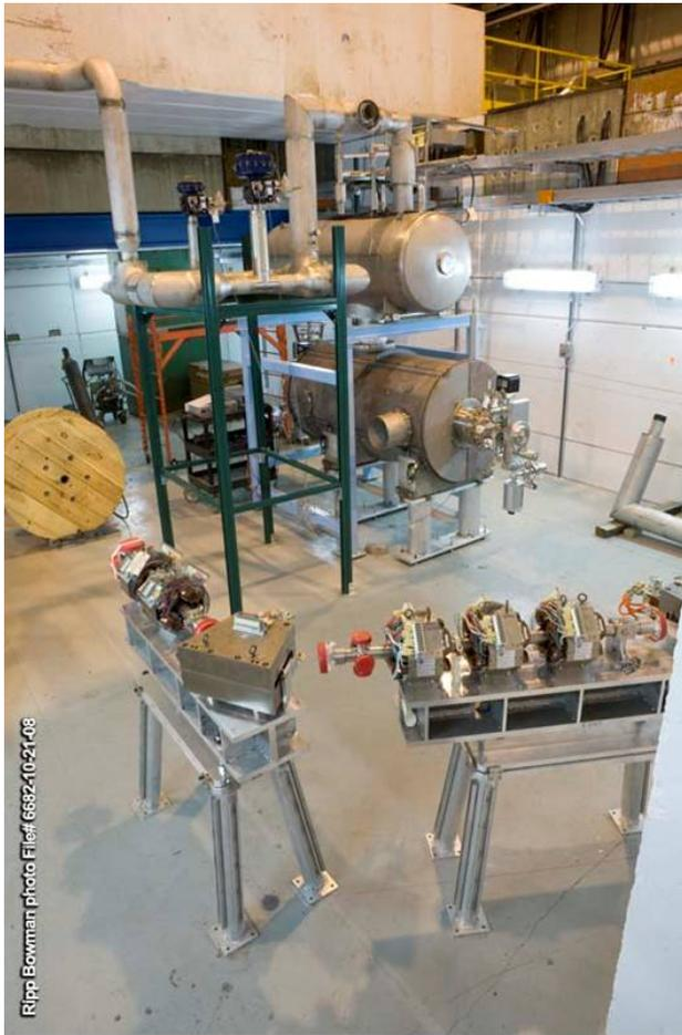
Figure 2: The cryomodule and liquid helium ballast tank installed in the ERL blockhouse.
