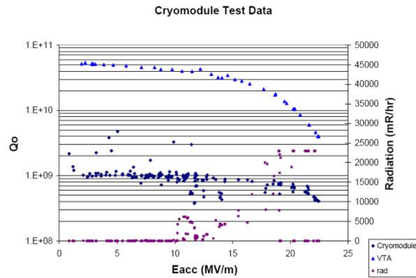
Figure 4: The preliminary test data from the cryomodule including radiation measurements presented along with the previous VTA measurements.
