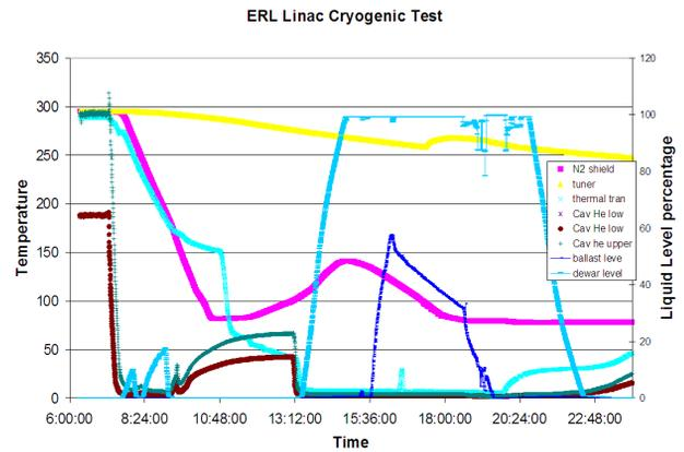
Figure 3: A summary of some of the relevant data from the first cryogenic cool-down of the cryostat.
