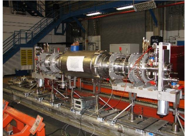
Figure 1: The ERL accelerating cavity hermetic string assembly shown before installation into the cryomodule.
