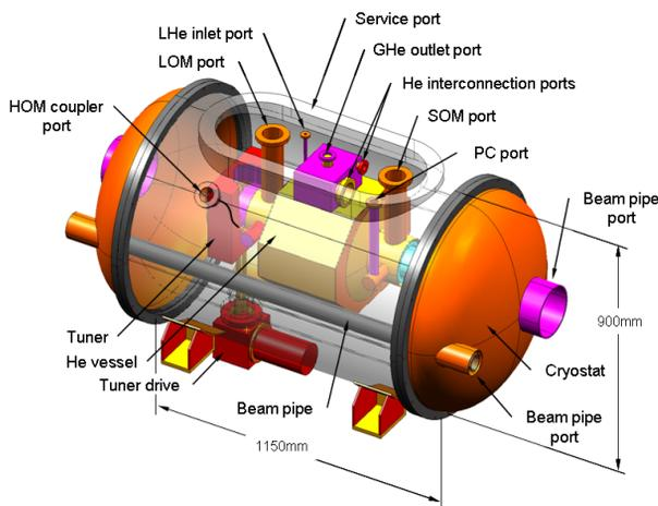
Figure 4: Schematic of the LHC Crab Cavity cryostat.
