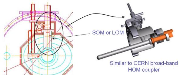
Figure 5: Possible design of the SOM/LOM couplers
