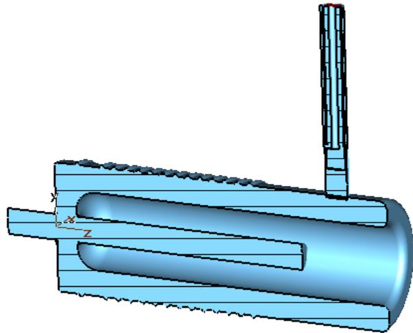
Figure 1: The 56 MHz SRF cavity shape in CST MicroWave Studio (MWS) simulation. The fundamental damper port is in the picture.
