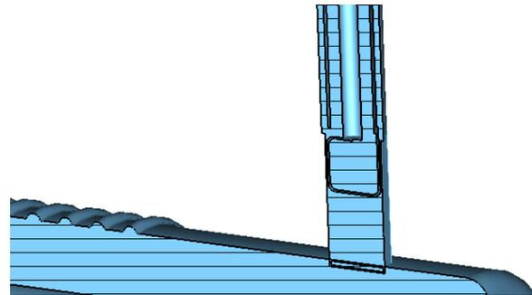
Figure 2: The enlarged fundamental mode damper picture. The fundamental mode damper is recessed by 10 cm from the cavity surface. The rectangular waveguide shape opening is extended and followed by a circular open port.
