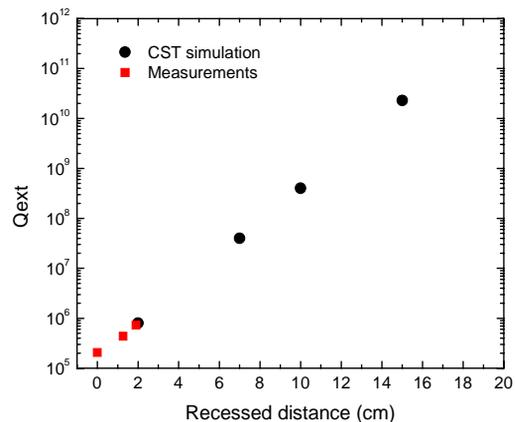
Figure 4: The external Q as a function of the fundamental mode damper location (the damper is recessed with respect to the cavity surface). Black dots represent the MWS simulation, and red squares represent the prototype measurement.
