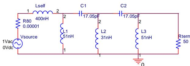
Figure 5: A new HOM filter circuit model.
