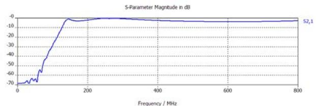
Figure 6: The MWS simulation result of the HOM filter.
