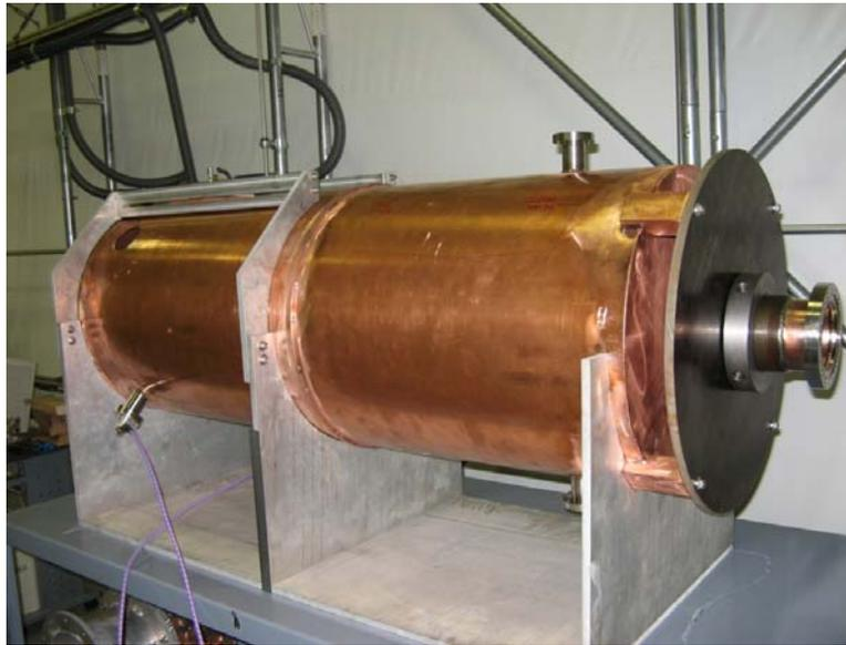
Figure 3: The prototype copper cavity.
