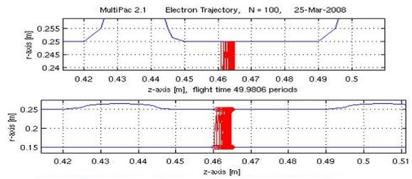
Figure 8: Multipacting trajectory with 4 cm gap between the ripples.
