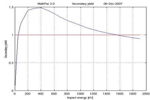
Figure 2: Secondary yield for niobium as a function of the electron impact energy in eV.
