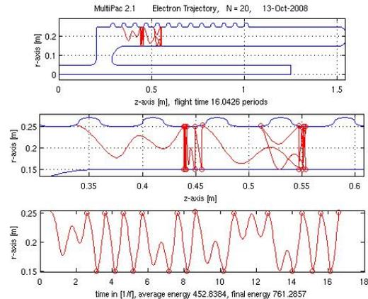
Figure 9: Discontinuities in the resonant electron's trajectory with gap 2 cm between ripples, even for only 20 impacts.
