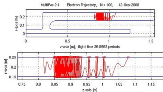
Figure 5: Electron trajectories for a peak surface electric field of 50 kV/m.
