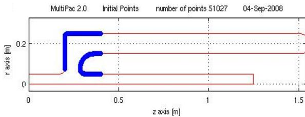
Figure 4a: Points between 20-40 cm where initial electrons were generated to cause multipacting.
