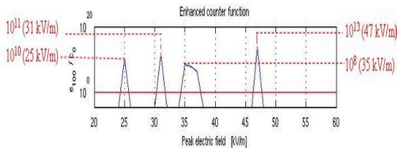
Figure 4b: Enhanced counter function for 100 electron impacts for the zone 20-40cm of the cavity.
