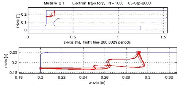
Figure 4d: Electron trajectory in two-point multipacting at 31 kV/m.
