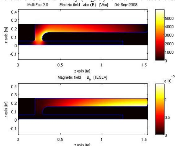
Figure 3: Electric and magnetic field distribution inside 56 MHz QWR cavity.
