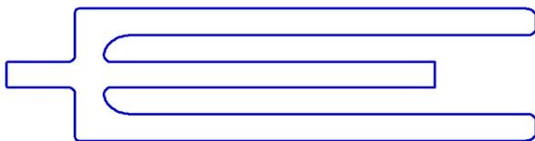
Figure 1: Outline of the 56 MHz RF Quarter Wave Resonator in 2-Dimension without coupler and dampers.
