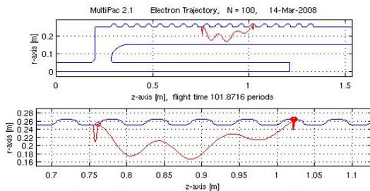
Figure 7: Stable trajectories of electrons inside a 3 cm wide ripple.
