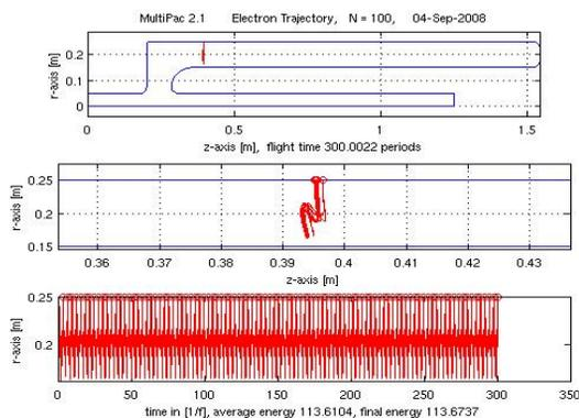
Figure 4c: Electron trajectory in single-point multipacting at 25 kV/m. The top figure represents the trajectory of the electron in (r, z) coordinates, the middle one is an expanded plot of a part of the top one, and the bottom plot illustrates the electron trajectory in (r, t) coordinates where t is the time in rf periods. The circles indicate the impacts on the walls of the cavity.
