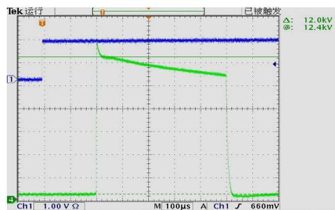
Figure 4: Pulse of the 12 kV solid switch cell module.
