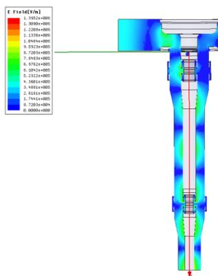
Figure 2: E-field of the KEK STF baseline high power input coupler with two choke structures.
