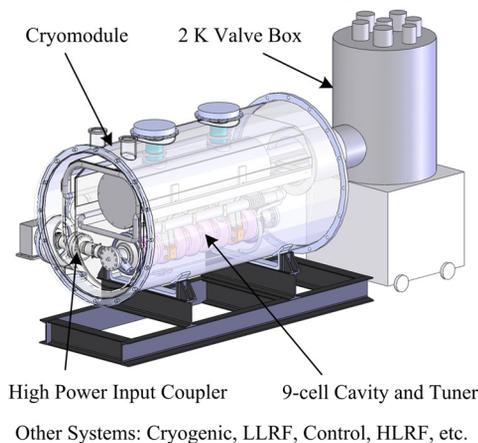
Figure 1: Layout of the IHEP 1.3 GHz SCRf Accelerating Unit
