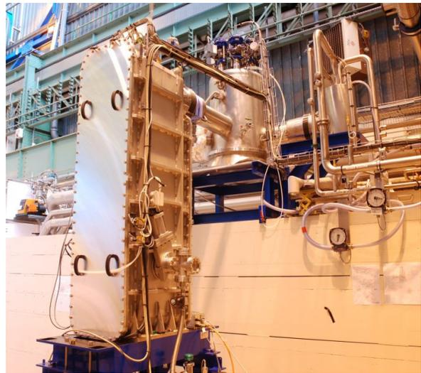
Figure 1: Cryomodule inside the test stand, connected to the valves box. RF coupler is not shown.
