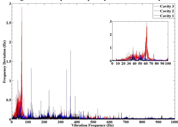
Figure 5: Cavity RF frequency deviation spectrum.
