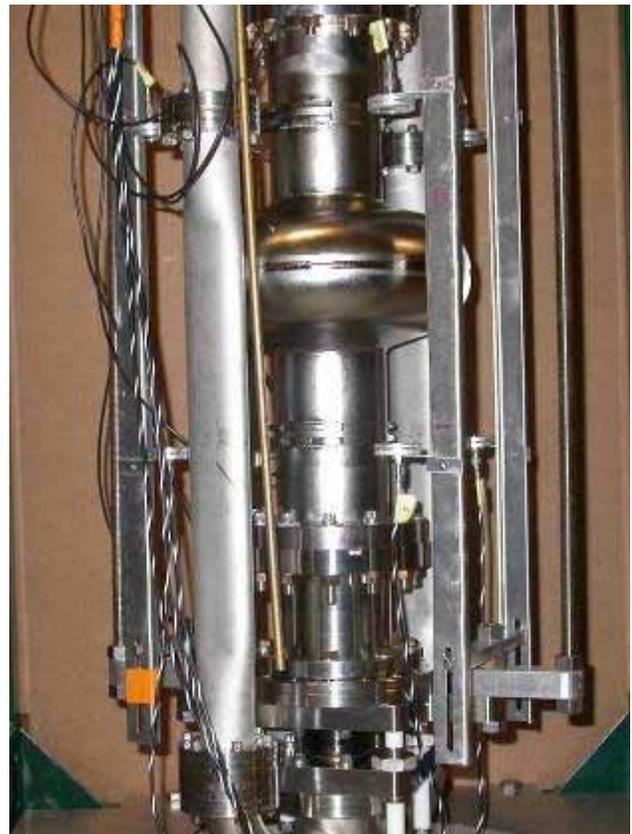
Figure 3: A single-cell cavity ready for testing. Six of the eight oscillating superleak transducers are visible.
