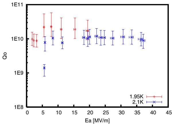
Figure 2: 5-Cell cavity vertical test results after baking at 120°C for 48 hours. During the initial pumping down to 1.95 K, the cavity reached 20 MV/m. After a subsequent helium transfer and continued pumping back down below the lambda point, the cavity reached a maximum accelerating field of 37.3 MV/m. The cavity was limited by a thermal quench.
