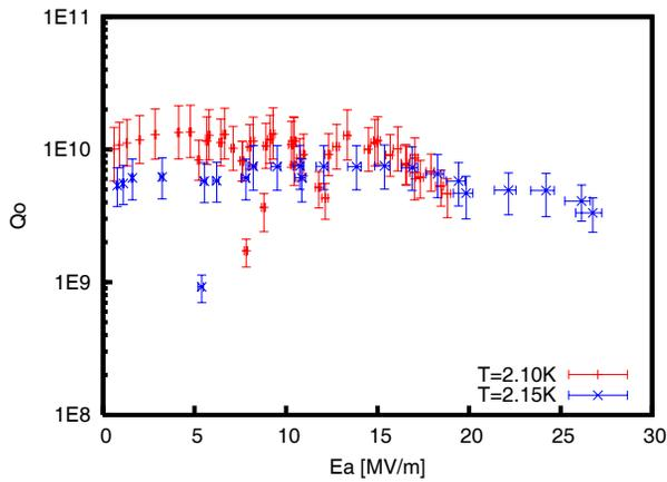
Figure 1: 5-Cell cavity vertical test results. Processing events were seen at low fields and the cavity was limited by field emission: 18.8 MV/m during the first test and 26.8 MV/m during the second test.
