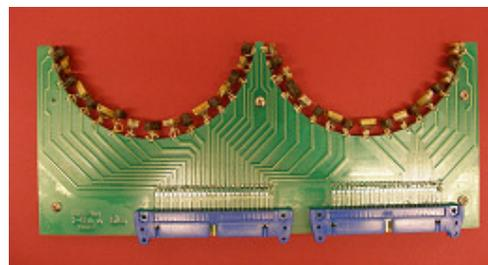
Figure 4: Temperature mapping thermometer board. A thermometer board for two cells containing 34 Allen-Bradley 120Ω resistive thermometers. The light colored thermometers have a G10 housing while the dark thermometers have a molded Stycast housing.
