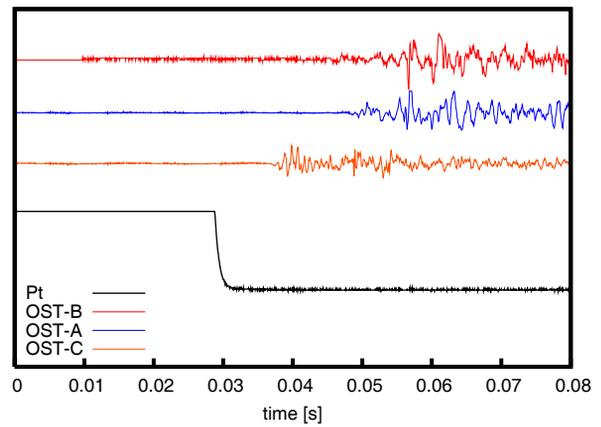
Figure 3: 5-Cell quench captured with OSTs. The transmitted power  $P_t$  drops to zero in 3 ms as the cavity stored energy is dissipated at the defect location. The OSTs' responses are delayed by the arrival time of the second sound wave front, traveling radially away from the defect at a speed of 20.3 m/s.
