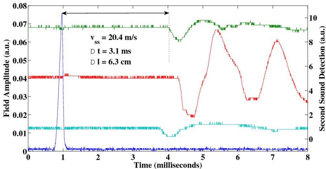
Figure 4: OST data for a single quench event. The lower trace is cavity field amplitudes, and the three upper traces are OST signals. The small time discrepancy between measured arrival times correspond to different OST positions. The OSTs all found the cavity quench to be a global event.
