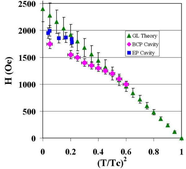
Figure 2: Graph of  $H_{sh}$  vs  $(T/T_c)^2$ , where  $T$  is the bath temperature. The green triangles are the GL prediction  $H_c^{RF}(T) = 1.2H(0)[1 - (T/T_c)^2]$ , with  $H(0) = 2000$  [2]; error bars of 10% have been included to correspond with the uncertainty in  $c_{sh}$ . The pink diamonds are the BCP cavity results [3]. The blue squares are the most recent EP cavity results. Error bars of  $\pm 5\%$  have been included corresponding to calibration uncertainty.
