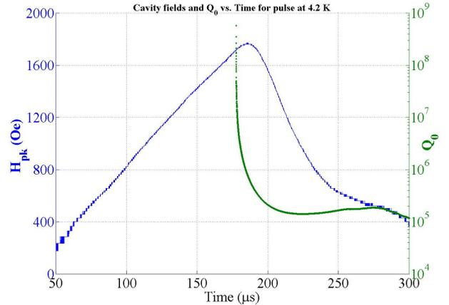
Figure 3: Plot of  $H_{pk}$  (blue line) vs. time and  $Q_0$  (green dots) vs time at 4.2 K. The RF power pulse lasted from 25 - 275  $\mu s$  on the trace. The cavity becomes normal conducting at a peak field of 1760 Oe. Prior to this time, the  $Q_0$  of the cavity is too high to be measured by methods used in pulsed operation.
