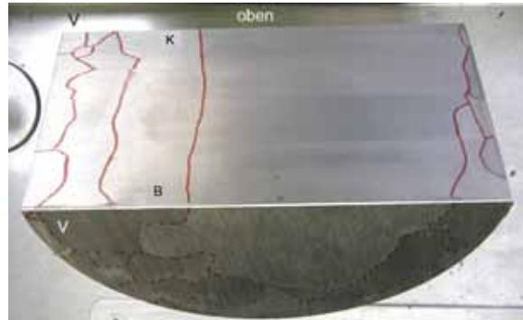
Figure 1: Example of single crystals growth in the ingot of ca. 300 mm diameter of Co. W. C. Heraeus.
