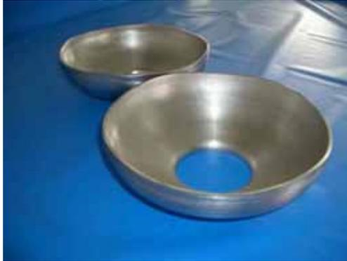
Figure 2: Discs of the single crystal with crystallographic orientation (100) after deep drawing.
