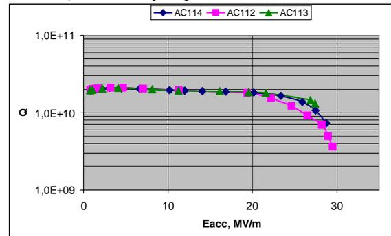
Figure 3:  $Q(\text{Eacc})$  of the cavities AC112- AC114; first test after about 100  $\mu\text{m}$  rough BCP, annealing at 800°C for 2h followed by a fine BCP of 20  $\mu\text{m}$ .
