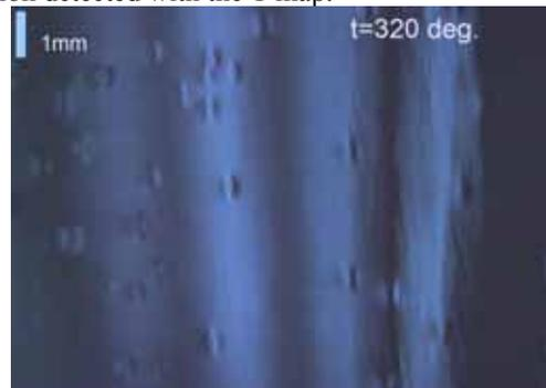
Figure 6: Example of craters seen on optical inspection image of the inner cavity AC114.
