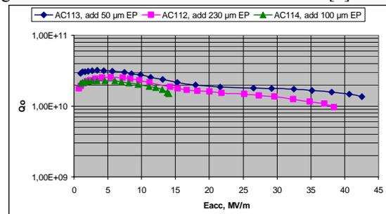
Figure 4:  $Q(\text{Eacc})$  of the cavities AC112- AC114 after additional EP treatment.
