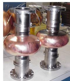
Figure 4: Two Nb Cu0.15%Zr clad cavities in preparation for tests.
