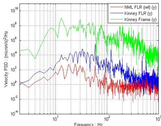
Figure 7: NML vertical PSD velocity Kinney test.
