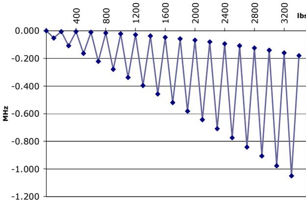
Figure 3: Cycling loads and frequency shifts of the cavity during the operation of inelastic tuning.
