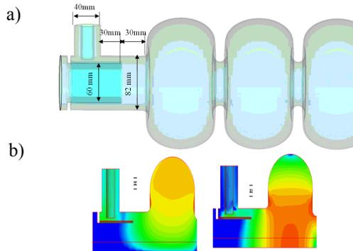
Figure 4: The coaxial coupler unit layout that preserves the axial symmetry of the accelerating channel (a); and rf field pattern (b).
