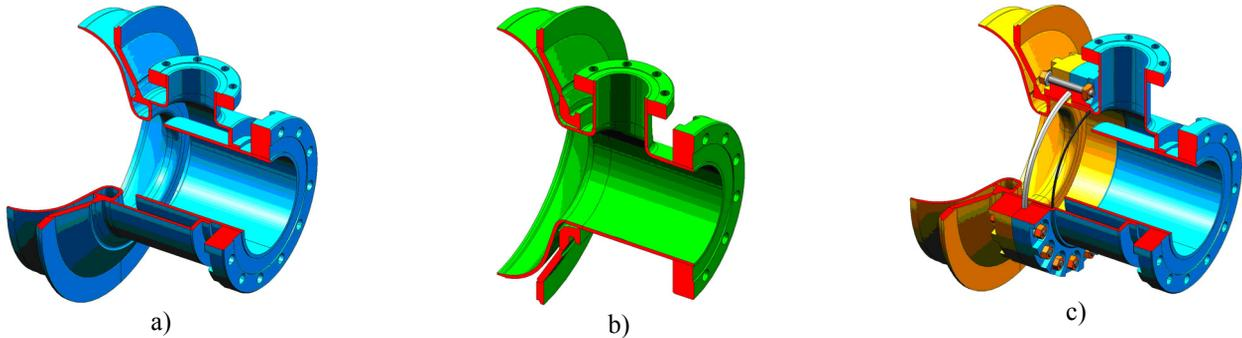
Figure 8: The 3D model of the mechanical design of the non-detachable quarter-wave coupler (a), standard of the coupler unit (b), and the detachable quarter-wave coupler(c).
