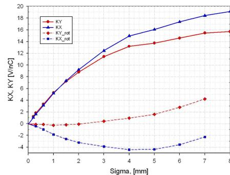
Figure 2: The horizontal (solid blue) and vertical (solid red) kick dependence versus the bunch length  $\sigma$ . Dashed curves show the kick dependences for the upstream coupler rotated by  $180^\circ$  versus the axis.
