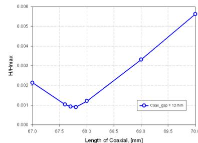
Figure 6: The magnetic field behavior in the cavity corner (see Fig. 5) versus the cavity length. H<sub>max</sub> is the maximal field in the cavity. Multipactoring analysis was done using Analyst code [11], no multipactoring was found in the coaxial.
