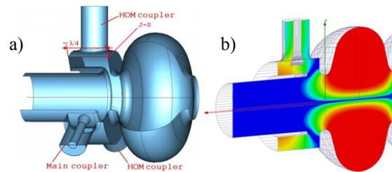
Figure 5: The idea of a resonance quarter-wave coupler unit (a) and rf field pattern (b).
