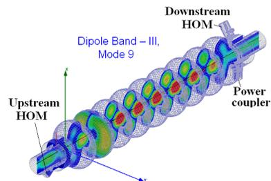
Figure 7. HFSS model of a standard 9-cell TESLA cavity with the two quarter-wave coupling units containing a power coupler, and HOM couplers.
