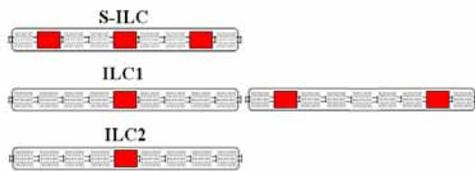
Figure 4: Modified Type-4 ILC cryomodule schematics. The cryomodule in S-ILC section contains three quads in the positions of 2d, 5<sup>th</sup>, and 8<sup>th</sup> cavities, and six 11-cell cavities. ILC1 has the two different quad location: in 5<sup>th</sup> position, and in 2d and 8<sup>th</sup> positions.
