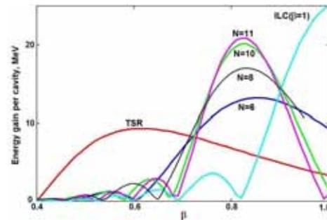
Figure 7: The energy gain per cavity versus  $\beta$  for the  $\beta=0.81$  cavities with different number of cells. The surface peak electric field is 50 MV/m.
