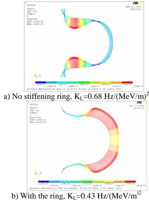
Figure 6: Mid cell deformations caused by the Lorentz force. Wall thickness is 3 mm.
