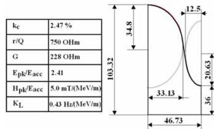
Figure 5: Parameters and dimensions (in mm) of the optimized regular cell. Lorentz factor  $K_L$  is given for optimal stiffening ring.
