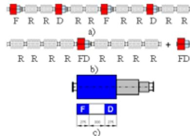
Figure 2: The cryomodule scheme: (a) - basic design that contains four lenses and eight 8-cell cavities; (b) proposed Type-4 ILC cryomodule containing eight 11-cell cavities and doublet, and additional doublet in a separate cryostat; c) schematic of the doublet.
