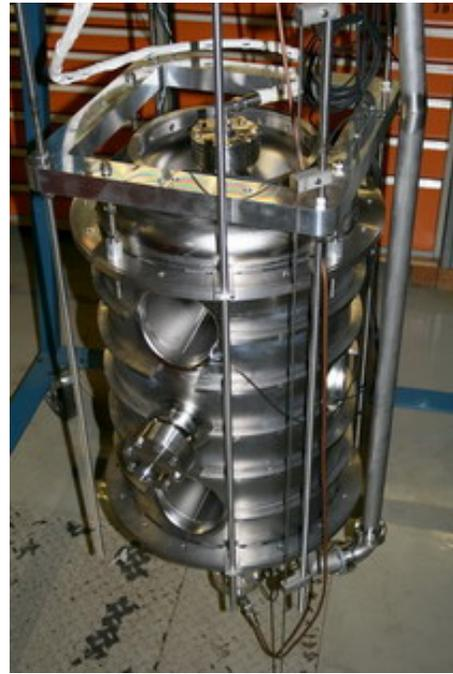
Figure 5: Triple-spoke cavity at FZJ test stand..
