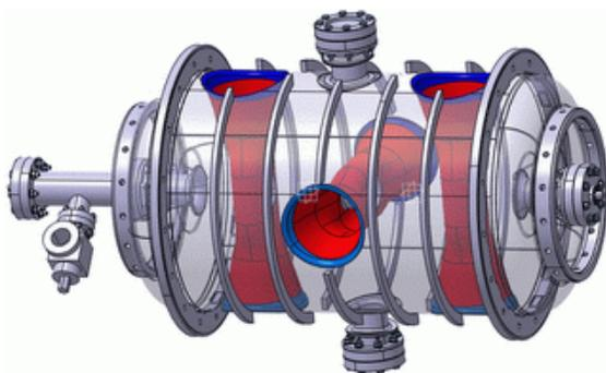
Figure 1: 3D view of triple-spoke cavity.
