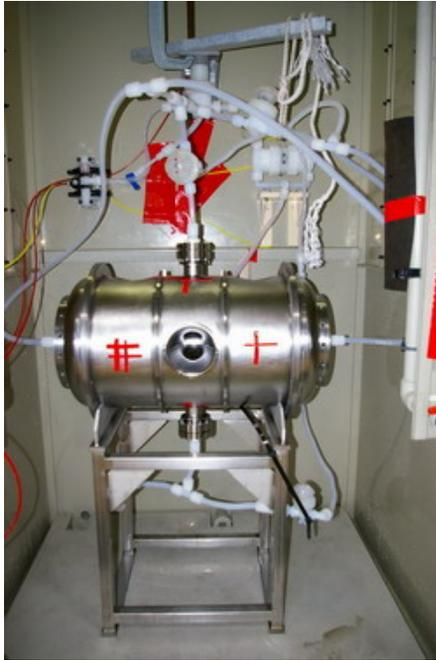
Figure 4: BCP installation at CEA-Saclay.
