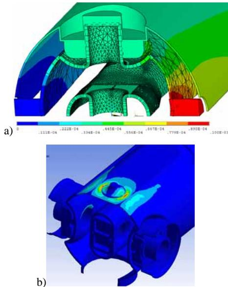
Figure 3: Cavity tune by wall deformation (a – displacements, b – stresses von Misses).
