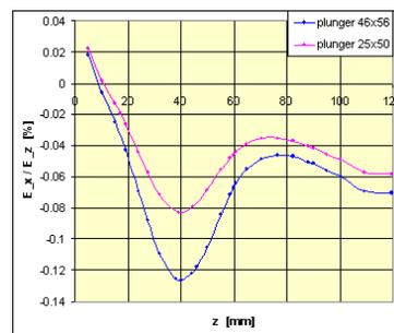
Figure 7: Cavity transverse component of accelerating field along beam path.
