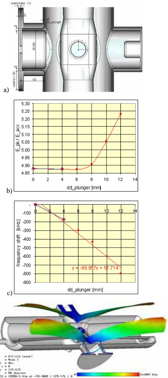
Figure 4: Capacitive tuner optimisation.
