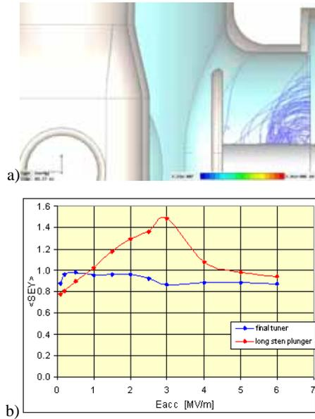
Figure 5: Capacitive tuner housing multipactor simulations.
