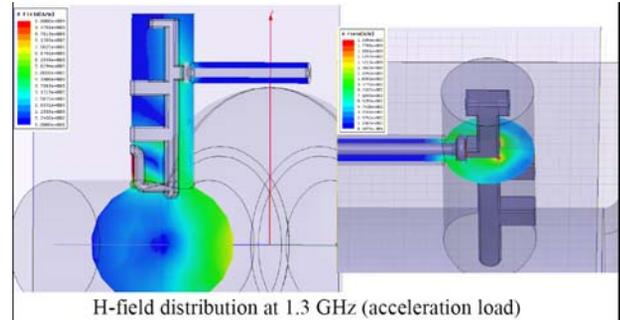
H-field distribution at 1.3 GHz (acceleration load)
