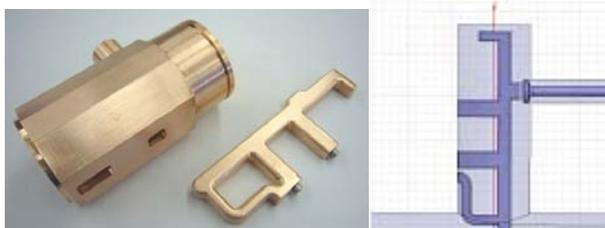
Figure 5: Two stub HOM coupler.
