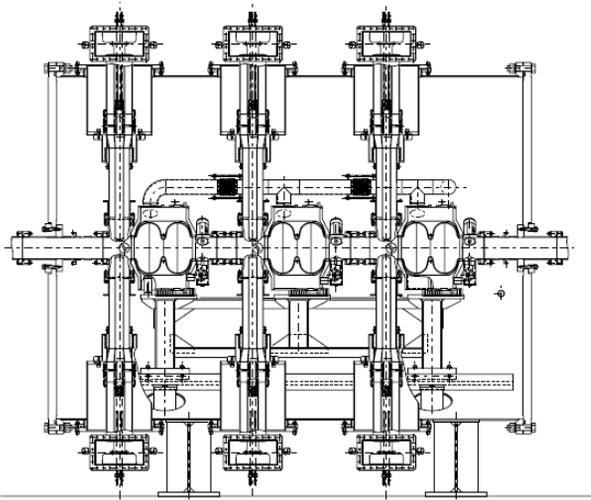
Figure 8: Injector cryomodule.
