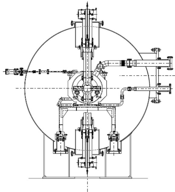
Figure 9: Injector cryomodule.
