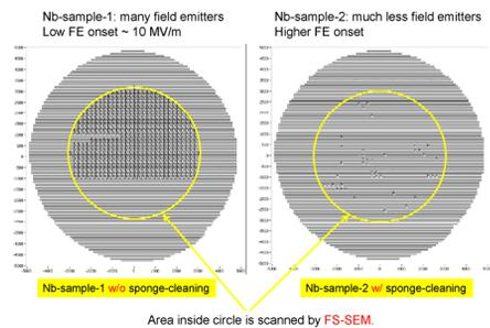
Figure 4: Results of SFEM analysis. Left-hand side: Nb-sample-1 w/o sponge-cleaning. Right-hand side: Nb-sample-2 w/ sponge-cleaning. Each horizontal line corresponds to a scan by SFEM. Each peak corresponds to a field emitter.
