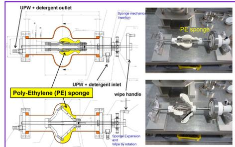
Figure 5: Left-hand side: drawings of proto-type sponge-cleaning tool for single-cell cavity. Right-hand side: pictures of sponge-cleaning tool.
