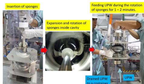
Figure 6: Test of proto-type sponge-cleaning tool.
