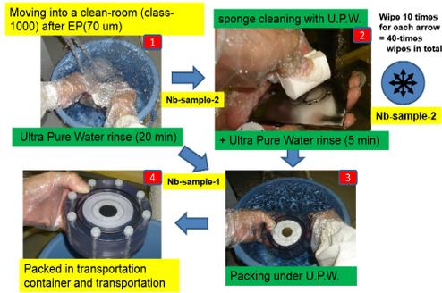
Figure 3: Nb-sample-1 was processed through 1) UPW rinse, 3) packing, and 4) transportation. Nb-sample-2 was processed through 1) UPW rinse, 2) sponge-wipe + UPW rinse, 3) packing, and 4) transportation.
