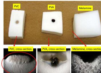
Figure 1: 20 ml of EP acid (no dilution) was dropped on PVC, PVA and melamine samples. PVC and melamine samples were melted completely and pits were made on the surface. On the other hand, a bump was made on the PVC surface from the expansion of sponge texture.
