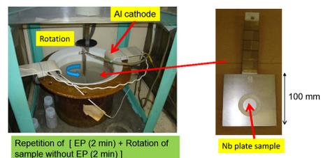
Figure 2: Setup of EP in laboratory. EP condition: Voltage = 8 ~ 13 V, Current = 3 ~ 23 A with oscillation, EP acid temperature = 25 ~ 50  $^{\circ}\text{C}$  without cooling system.
