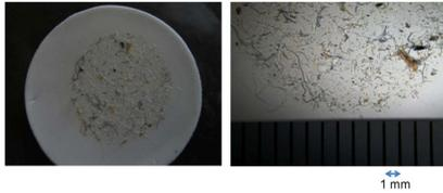
Figure 7: Pictures of residuals on the filter-paper. The residuals include fibers and particles.
