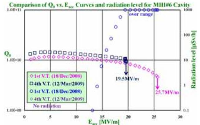
Figure 5:  $Q_0 - E_{acc}$  curves (square, diamond) and the radiation level (circles) for MHI#6 cavity.
