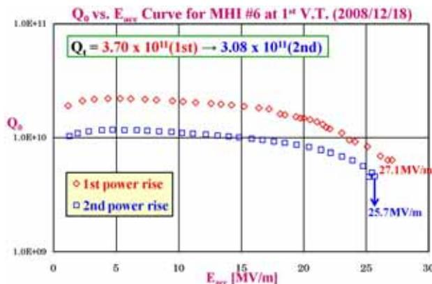
Figure 7:  $Q_0$  and  $Q_t$  degradation during one VT.
