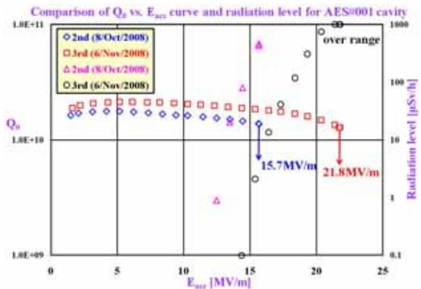
Figure 1:  $Q_0 - E_{acc}$  curves (square and diamond) and the radiation level (circle and triangle) for AES#001 cavity.
