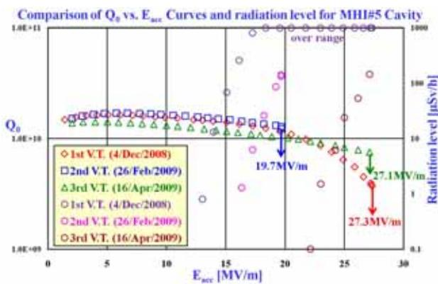
Figure 3:  $Q_0 - E_{acc}$  curves (square, diamond and triangle) and the radiation level (circles) for MHI#5 cavity.
