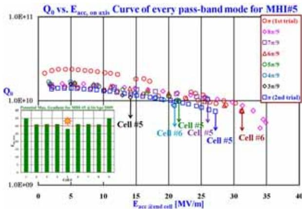
Figure 4:  $Q_0 - E_{acc@end cell}$  curves and achievable gradient for each cell (small figure) at 3<sup>rd</sup> test.
