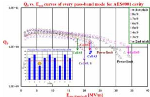
Figure 2:  $Q_0 - E_{acc @end cell}$  curves and achievable gradient for each cell (small figure) at 2<sup>nd</sup> test.
