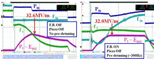
Figure 2: Observation of Lorentz detuning during the high power test without F.B. and the pre-detuning (left), and with them (right). Blue shows the klystron output, green shows the cavity phase and purple shows the cavity field.
