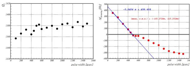
Figure 4: Result of the Loaded Q (left) and the detuning frequency (right) by the pulse shortening method. F.B. and Piezo are not used in this case.
