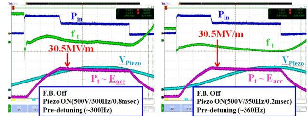
Figure 5: Compensation of the Lorentz detuning by Piezo. Light blue shows the drive pulse of Piezo.
