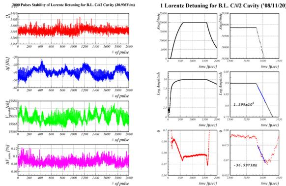
Figure 8: Result of the pulse stability test around 30MV/m. Left shows the time trend and right shows the status of one pulse.
