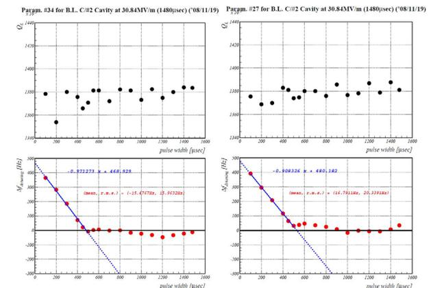
Figure 6: Examples of Piezo compensation measured by the pulse shortening method around 30MV/m.
