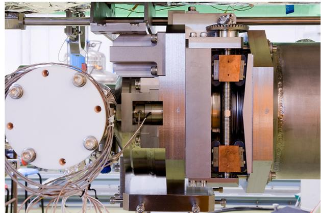
Figure 1: Slide-Jack tuner at STF Cryomodule.
