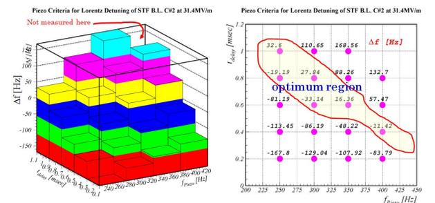
Figure 7: Optimum region of Piezo drive for the compensation of the Lorentz detuning. The vertical axis in the left is the detuning frequency. The numerical values in the right are the detuning frequency.
