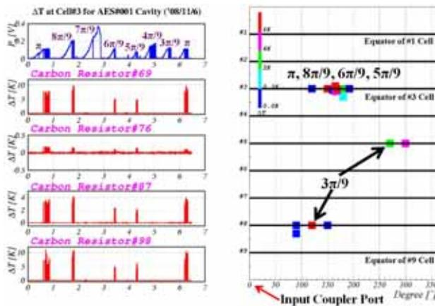
Figure 2: Trend graph and heating location from T-mapping result for AES#001 cavity at 3<sup>rd</sup> V.T.
