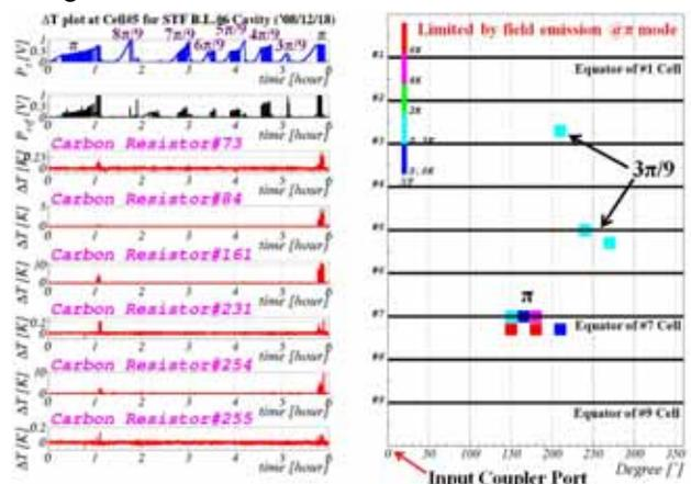
Figure 5: Trend graph and heating location from T-mapping result for MHI#6 cavity at 1<sup>st</sup> test.
