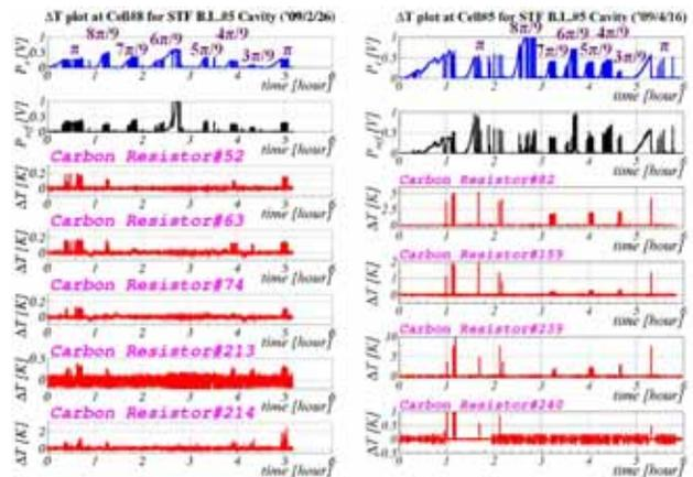
Figure 3: Trend graph of heating at 2<sup>nd</sup> (left) and 3<sup>rd</sup> (right) V.T. for MHI#5 cavity.
