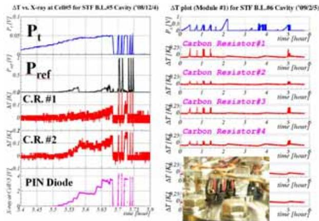
Figure 7: Example of the pre-heating before the thermal quenching (left) and the heating at the top flange (right).
