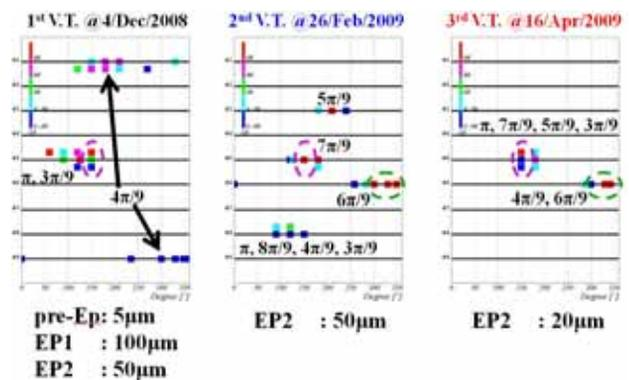
Figure 4: Changes of the heating location for MHI#5 cavity among three tests.
