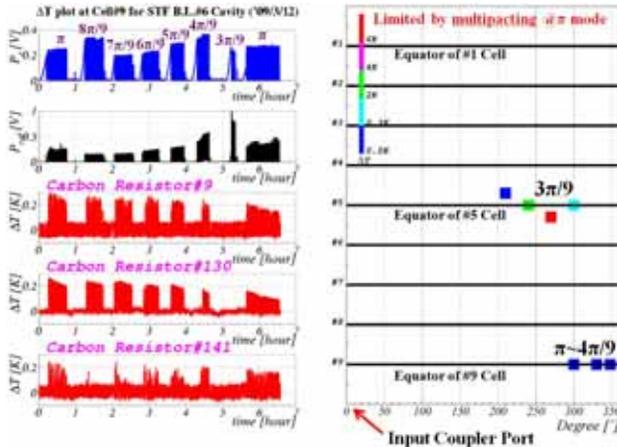
Figure 6: Trend graph and heating location from T-mapping result for MHI#6 cavity at 4<sup>th</sup> test.
