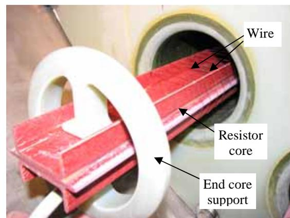
Figure 4: Resistor assembly with GPO-3 resistor core and G10 end core support.
