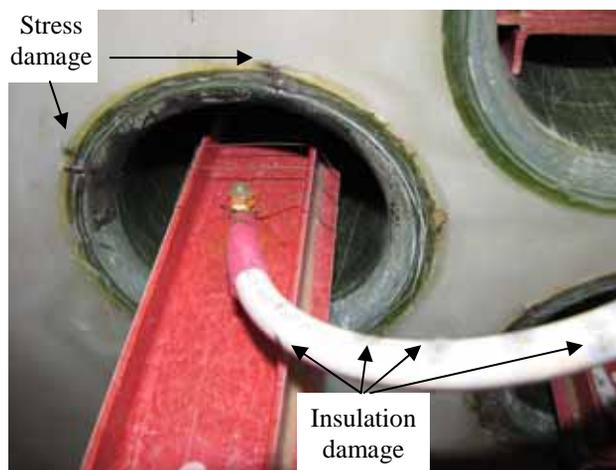
Figure 5: Electrical damage on silicone-insulated lead and stress damage at dielectric-to-dielectric interface.
