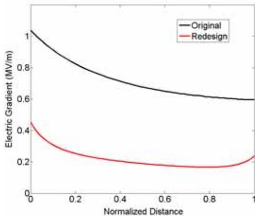
Figure 2: Electric field gradient through the peak electric field paths of the original and redesigned loads shown in Fig. 1.
