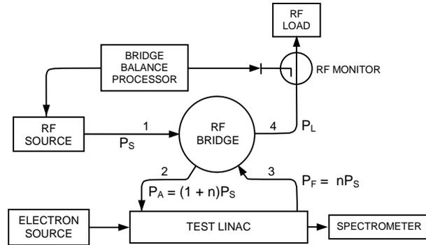
Figure 1: Typical four port RF bridge configuration for a resonant ring linac test facility using phase lock feedback control.
