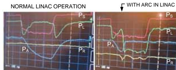
Figure 2: 50 ns/div waveforms showing, during a structure breakdown, rapid termination of the linac power ( $P_A$ ) and transmission of the source power ( $P_S$ ) to the load ( $P_L$ ). ( $P_R$  is the linac reflected power signal.)
