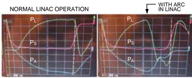
Figure 3: 20 ns/div waveforms of the fast redirection of source power to the load during a self-quenching breakdown in the structure.
