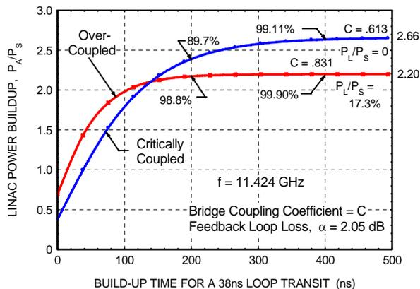
Figure 4: Comparison of linac power buildup for a critically coupled (C=.613) and an overcoupled (C=.831) resonant ring having a feedback loop loss of 2.05 dB.
