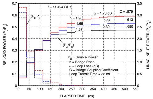
Figure 5: Linac input power ( $P_A/P_S$ ) buildup and load power ( $P_L/P_S$ ) decay for critically coupled resonant ring systems having bridge ratios of 1.98, 1.66 and 1.37.
