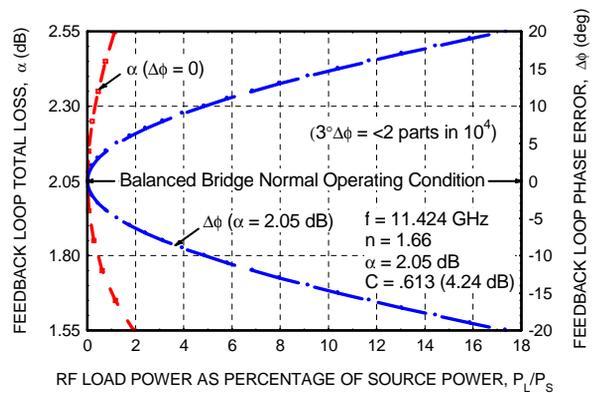
Figure 7: RF bridge load monitor computed response to power imbalance caused by a change in phase or attenuation of the linac feedback loop.
