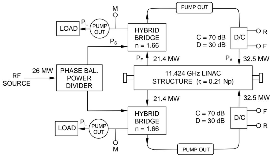
Figure 6: An 11.424 GHz dual resonant ring system with an embedded CLIC/KEK/SLAC (T18) linac structure showing the power distribution required for operation at an unloaded average accelerating gradient of 108 MV/m.
