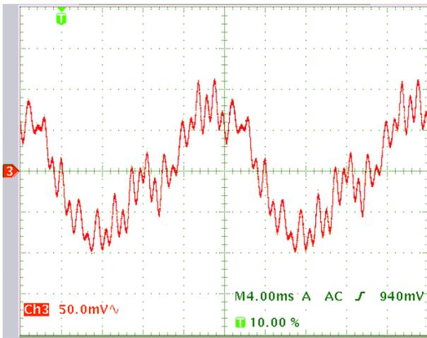
Figure 5: Measured ripple in the output voltage from the klystron power supply. Operating voltage: 40 kV, current: 6.4 A. Ordinate: output voltage (100 V/div; AC coupling), abscissa: time (4 ms/div.).
