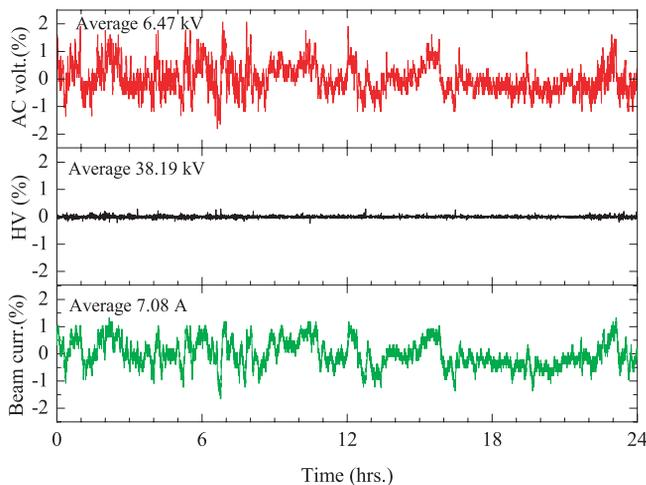
Figure 6: Stability in the high voltage of the new power supply during one day. Relative variations in the input AC voltage, in the DC high voltage, and in the klystron beam current are shown.
