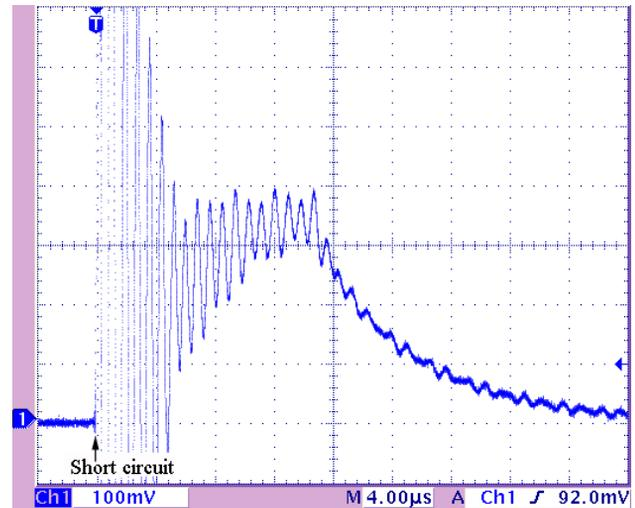
Figure 4: Result of the short circuit test. Ordinate: short-circuit current (10 A/div.), abscissa: time (4  $\mu$ s/div.).
