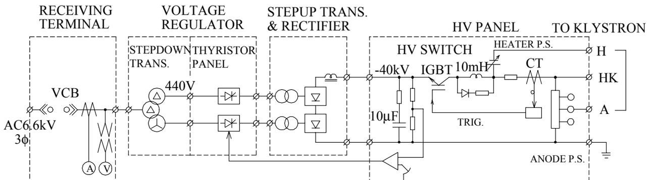
Figure 1: Block diagram of the new klystron power supply for the PF storage ring.
