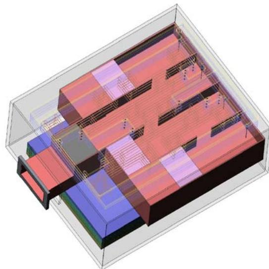
Figure 3: Waveguide RF power adder.
