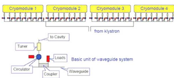
Figure 1: RF waveguide distribution of klystron based XFEL RF station.
