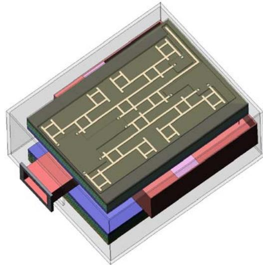
Figure 2: Strip line RF power adder.
