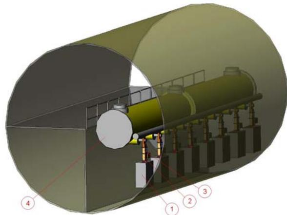
Figure 5: Accelerator module with Solid State High Power RF System in XFEL tunnel.
