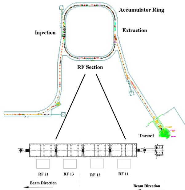
Figure 2: Layout of ring RF components.
