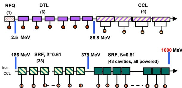
Figure 1: Layout of LINAC RF modules.
