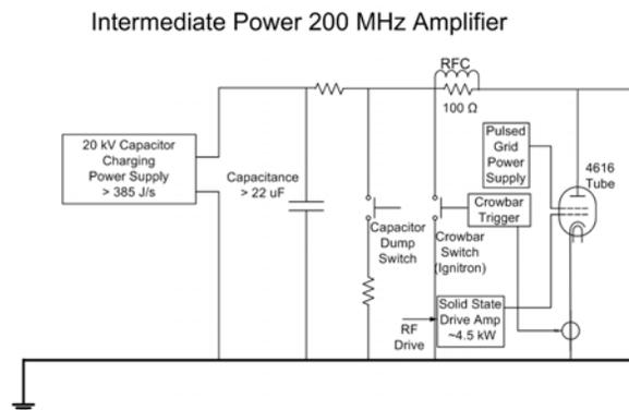
Figure 2: Intermediate amplifier.
