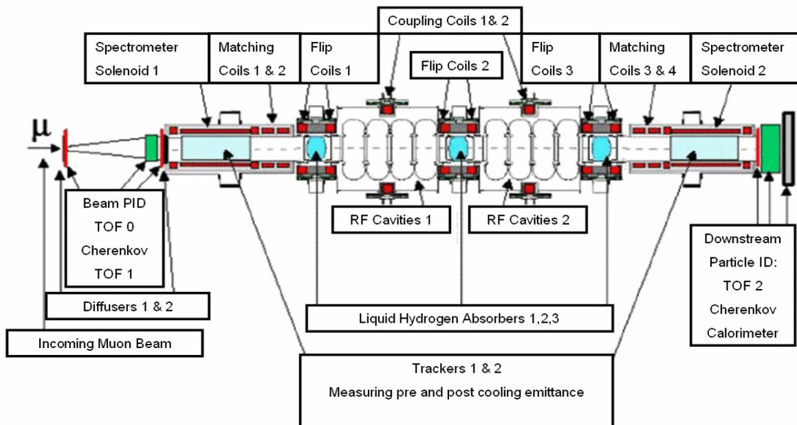
Figure 1: MICE cooling channel.
