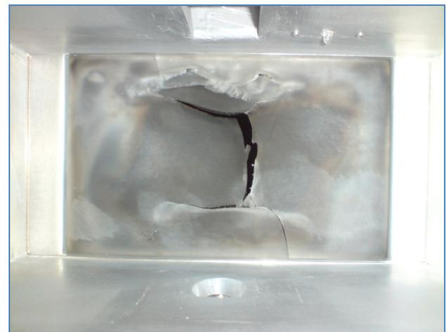
Figure 4: Booster Cavity 1 Window Failure.
