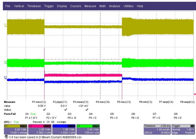
Figure 3: Beam dump procedure without amplitude loop constraint. The IOT forward power (dark green trace) is larger after the beam dump due to the cavity mismatch and loop counteraction. Light green trace is the reflected power, blue trace is the IOT collector current.
