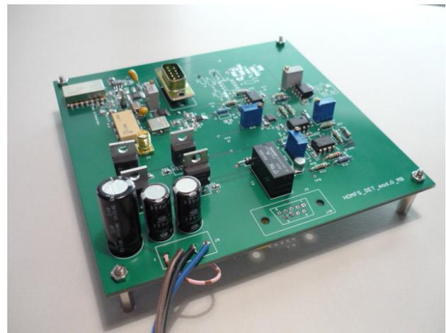
Figure 1: HOM detector board.
