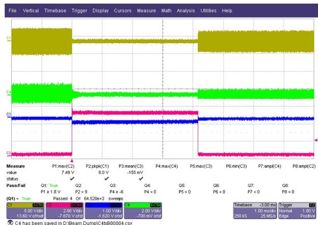
Figure 4: Beam dump procedure with amplitude loop constraint. Before the dump, the forward power is around 55 kW (accumulated current 330 mA). It backs to 28 kW, when the input power is applied to the cavity.
