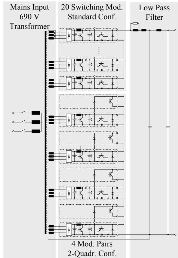
Figure 2: Modulator block diagram.
