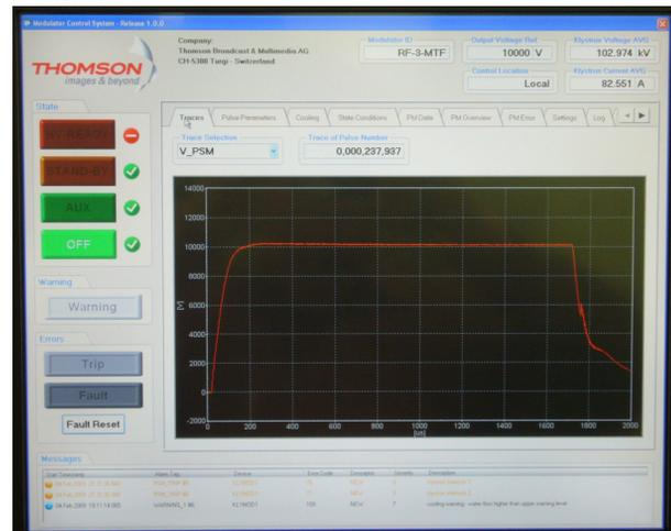
Figure 5: Control system screen with pulse waveform.
