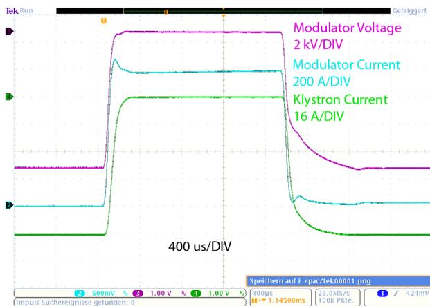
Figure 6: Pulse 10.5 kV / 1000 A.
