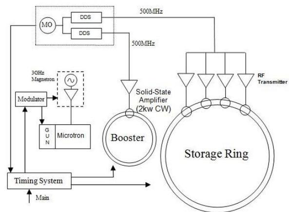
Figure 1: Simplified block diagram for RF distribution.
