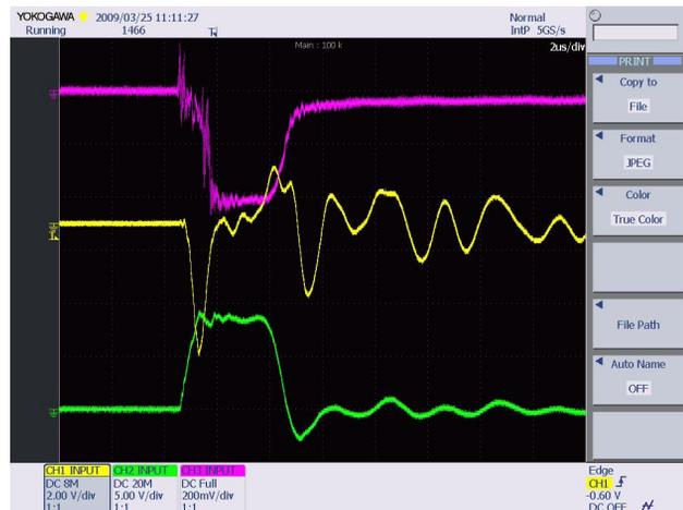
Figure 3: Microtron measured signals, RF pulse (upper), Gun current (middle), Magnetron current (lower).
