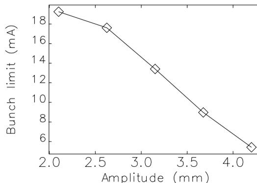
Figure 2: Bunch charge limit as a function of imparted horizontal betatron oscillation.
