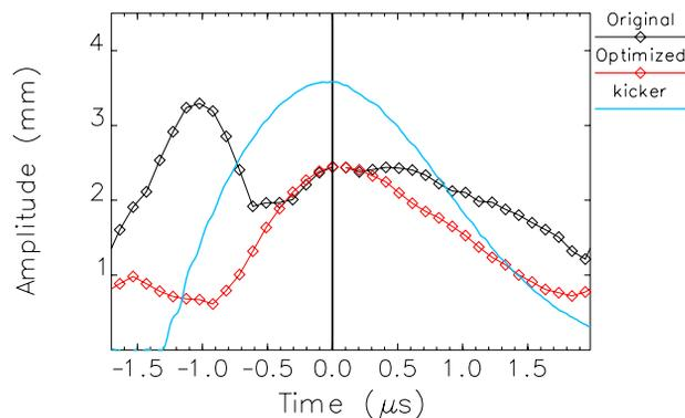
Figure 3: Betatron oscillations on non-targeted bunches as a function of time about the targeted bunch for two sets of sextupole settings. Ideal kicker waveform is superimposed.
