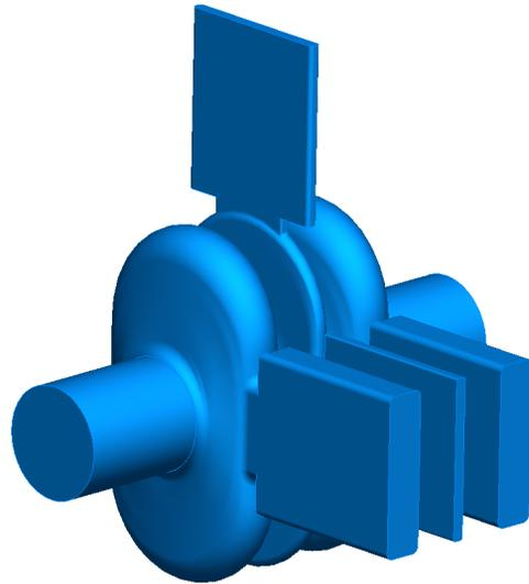
Figure 1: Geometry of a 3-cell cavity with horizontal cavity-mounted dampers on each cell. A vertical damper is located on the central cell to damp vertical dipole modes.
