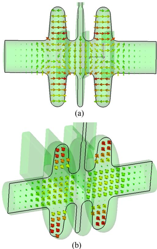
Figure 3: Field pattern for the  $\pi/2$  dipole mode: (a) electric field and (b) magnetic field.
