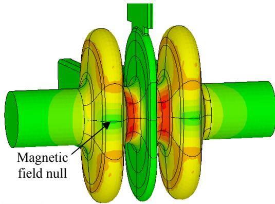
Figure 2: Magnetic field magnitude due to the  $\pi/2$  mode on the 3-cell cavity where the red and green colors represent the maximum and minimum field levels, respectively.
