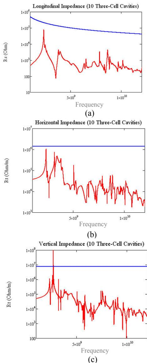
Figure 4: Impedance calculated by GdFidl for ten 3-cell cavities with matched port terminations: (a) longitudinal, (b) horizontal, and (c) vertical. The red plot represents the beam impedance and the blue line defines the APS stability limit.
