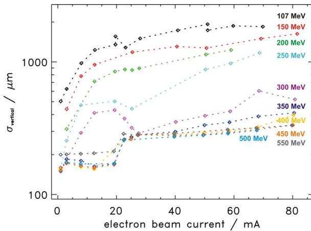
Figure 3: Vertical beam size ( $1\sigma = \text{rms}$ ) as function of the electron beam current at different beam energies (logarithmic scale).
