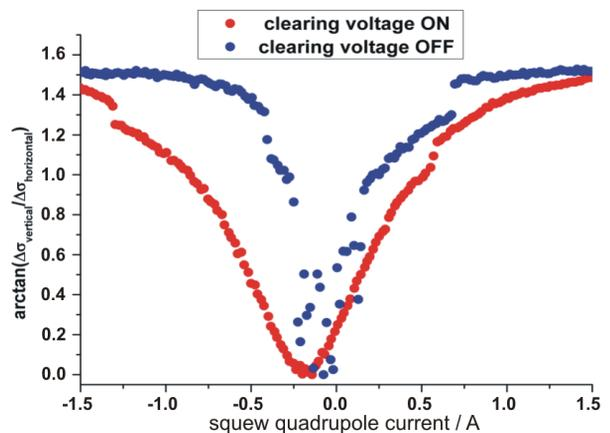
Figure 5: Measured at 630 MeV and 109 mA beam current the  $\arctan(\Delta\sigma_{\text{vertical}}/\Delta\sigma_{\text{horizontal}})$  versus squew quadrupole current is plotted with and without clearing voltage applied.  $\Delta\sigma$  are the changes of the source size due to the change of the quadrupole current.
