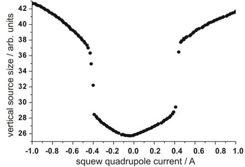
Figure 4: Vertical source size as function of the squew quadrupole current at a small value of the momentum compaction factor and at 630 MeV (clearing voltage on).
