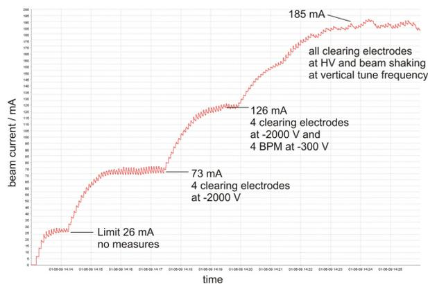
Figure 1: Current limits caused by beam ion interaction. While accumulating without any ion suppression the beam current saturates at low currents (26 mA). With each additional countermeasure applied the saturation current increases.
