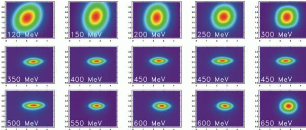
Figure 2: Beam images of a 100 mA beam taken on the ramp. Above 600 MeV coupling is enhanced by raising a squew quadrupole to improve Touschek lifetime.
