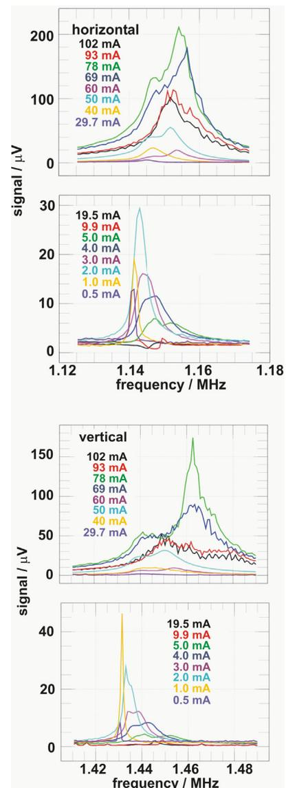
Figure 6: Transverse tune signals as function of the beam current at 630 MeV. Top: horizontal, bottom: vertical tune line; the beam current is coded by different colours.
