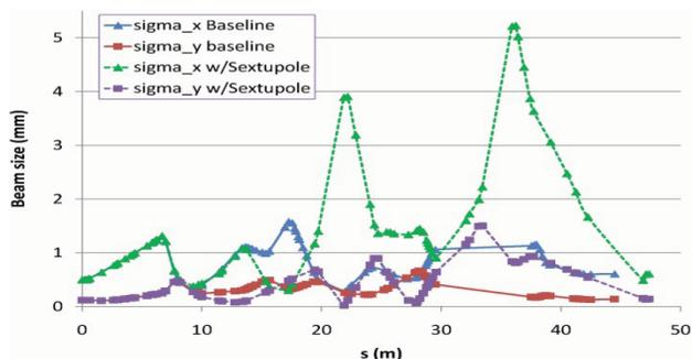
Figure 4: Beam Sizes through BSR transfer line for both injection options.
