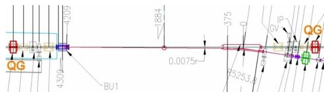
Figure 2: Booster injection straight. The pulsed septum is in red at 0 m. The injection kicker is labeled BU1.
