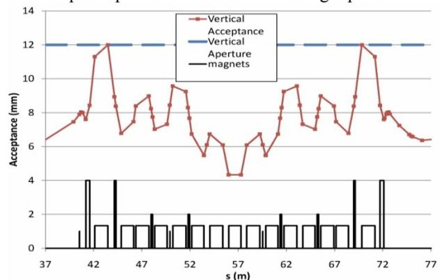
Figure 6: Vertical acceptance for one booster superperiod. The aperture limit is in the first horizontally defocusing dipole.
