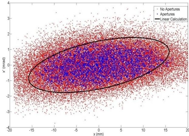
Figure 3: Horizontal phase space acceptance. The black ellipse is calculated from the Twiss parameters, the blue dots are a simulation with apertures, the red dots are a simulation without apertures.
