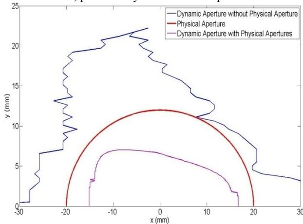
Figure 7: Dynamic Aperture of CD2 booster lattice shown with the physical aperture.
