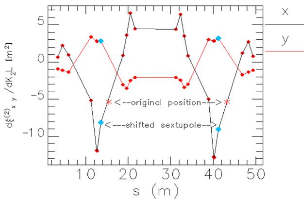
Figure 2: Sensitivity of the 2<sup>nd</sup> order chromaticity per unit of sextupole strength change ( $\Delta K_2L$ ). The diamonds represent sextupoles.
