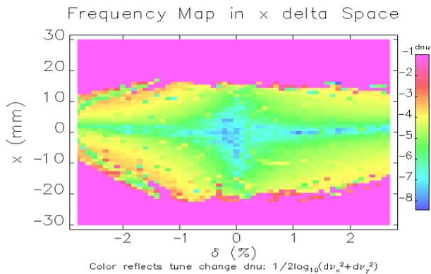
Figure 7: Diffusion weighted frequency map in  $(x, \delta)$  space.
