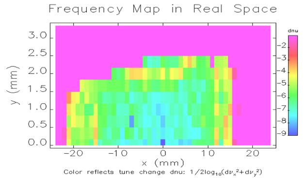
Figure 8: Diffusion weighted frequency map in  $(x, y)$  space.
