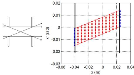
Figure 3 Determination of initial phase space area for forward tracking by four extreme rays.
