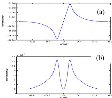
Figure 2: Quadrupoles (a) and sextupoles (b) vertical field component profiles on the mid-plane.
