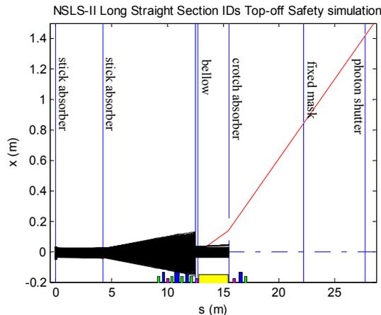
Figure 4: Beam trajectories (in black) in the normal condition. The central orbit of electron beam (blue dash line) is chosen as the reference, red solid line is the photon beamline centre, and blue solid lines are collimators.
