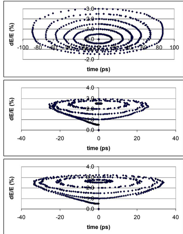
Figure 4. Longitudinal motion at horizontal tune of 9.78 and  $\chi_x/\chi_y = 2/2$ . Above:  $\alpha_c = 7.0 \times 10^{-5}$ . Motion is stable up to  $dE/E \approx 1.3\%$ . Middle:  $\alpha_c = 0.83 \times 10^{-5}$ . Motion is stable up to  $dE/E \approx 0.2\%$ . Bottom:  $\alpha_c = 0.32 \times 10^{-5}$ . Motion is stable up to  $dE/E \approx 0.05\%$ .
