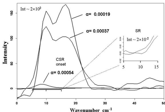
Figure 5. THz radiation intensity at various momentum compactions ( $\alpha$  in this figure). Inset figure shows non-CSR intensity.
