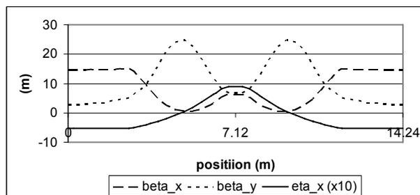
Figure 1. Machine functions (1 cell) for the initial CSR setup.
