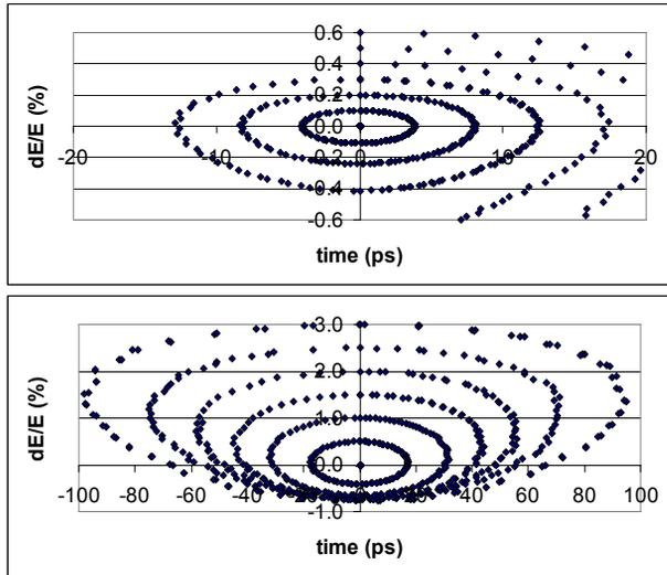
Figure 3. Longitudinal motion at a horizontal tune of 10.05, with  $\alpha_c = 6.8 \times 10^{-5}$ . Top:  $\chi_x/\chi_y = 2/2$ . Motion is stable up to  $dE/E \approx 0.3\%$  (compare to figure 2). Bottom:  $\chi_x/\chi_y = 4/2$ . Motion is stable up to  $dE/E \approx 3.0\%$ .
