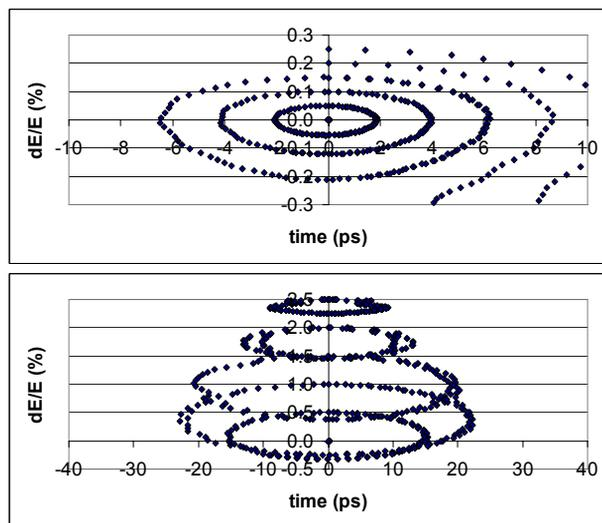
Figure 2. Longitudinal phase space tracking at different electron energies ( $dE/E$ ) for  $\alpha_c = 6.7 \times 10^{-5}$  at the nominal tunes. Top:  $\chi_x/\chi_y = 2/2$ . Motion is stable up to  $dE/E \approx +0.15\%$ . Bottom:  $\chi_x/\chi_y = 6/4$ . Motion is stable up to  $dE/E \approx 2.5\%$ . (Note: orbits appear to cross because this is a 2D slice of a 4D phase space.) In both cases the bunch lengths (from tracking) are effectively the same.
