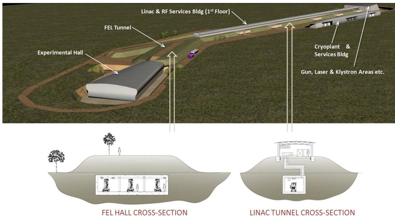
Figure 3: Architectural layout of the NLS facility.
