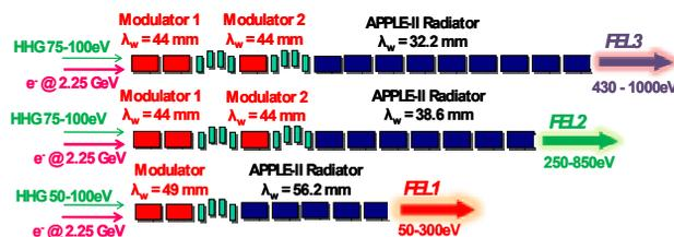
Figure 2: Schematic of the harmonic cascade FEL scheme.
