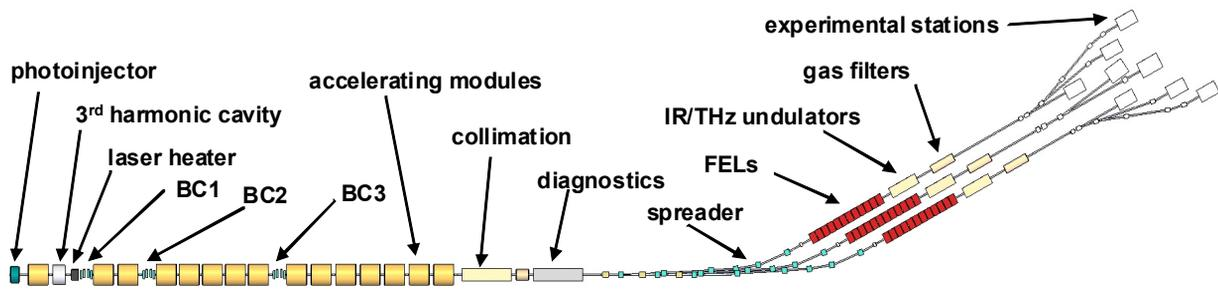
Figure 1: Schematic layout of the NLS facility.
