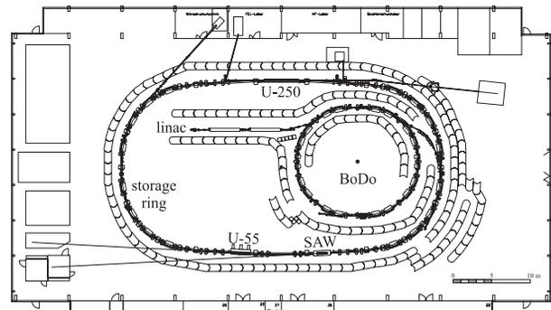
Figure 1: DELTA floorplan. The facility comprises a 60-MeV linac, a booster synchrotron (BoDo) and a 1.5-GeV electron storage ring, including three insertion devices (SAW, U-55, U-250).
