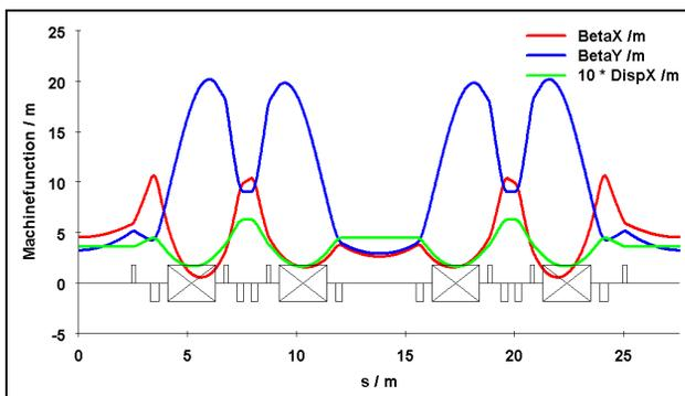
Figure 6: Beta functions for the modified ANKA storage ring optics.
