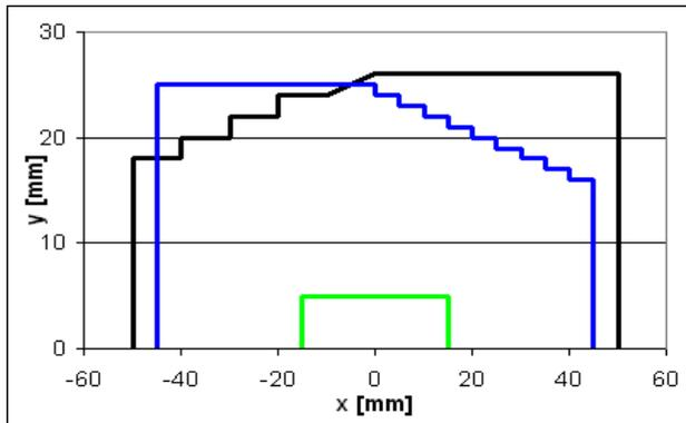
Figure 2: Dynamic aperture for 'eddy-current-sextupoles' only (black) chromaticity -5/-10. Chromaticity corrected to 1/1 (blue), and acceptance (green).
