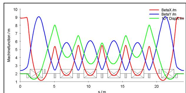
Figure 1: Beta functions for one quart of the ANKA full energy booster with vertical focussing gradient dipole.
