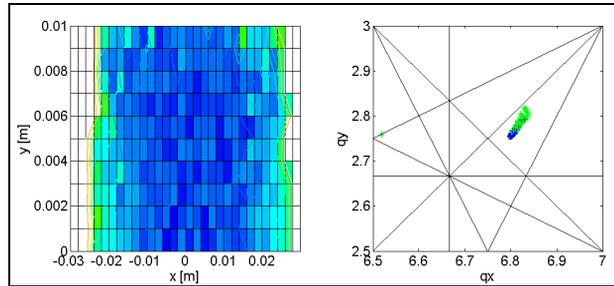
Figure 7: Dynamic Aperture of the modified ANKA storage ring optics and frequency map. Colour code for diffusion: red:  $> 10^{-3}$ , green:  $10^{-3} - 10^{-6}$ , blue:  $< 10^{-6}$ .
