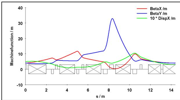
Figure 5: Beta functions for the booster to storage-ring transfer-line.
