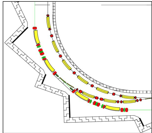
Figure 8: Layout of one quart of the modified ANKA storage ring and full energy injector.
