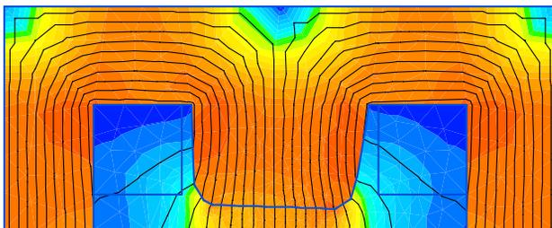
Figure 3: Magnetic field plot of the gradient magnet.
