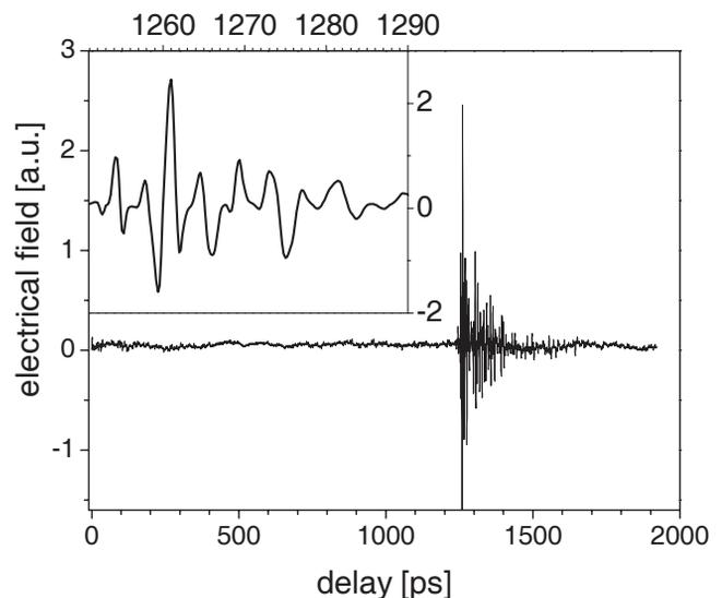
Figure 2: Electro-optical AC signal within the ZnTe crystal within the complete 2 nanosecond pulse-to-pulse separation and a magnification of the prompt signal of the THz pulse as inset.
