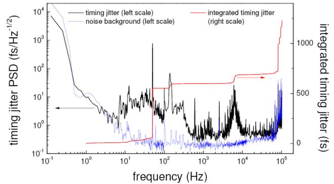
Figure 1: Spectral power of the phase noise of the pickup signal from the ring electrode compared to the reference signal from the bunch clock at 500 MHz together with the accumulated jitter below the given frequency. The synchrotron frequency is seen at 8.4 kHz contributing about 200 fs.
